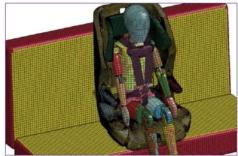
Hybrid III 6-year-old ATD in a forward-facing child restraint on the C/FMVSS bench in a finite element simulation
