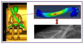
Pictured clockwise left to right: CIREN case MADYMO reconstruction with scaled 6-year-old ATD model seated in 3-point belt with backless booster; FE age-matched pediatric clavicle with stress distribution resulting from ATD shoulder belt contact loading in MADYMO reconstruction; X-ray of clavicle fracture from corresponding CIREN case
